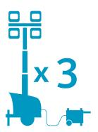
The HiLight E3+ has both IN and OUT connections for daisy chain capabilities, allowing up to 3 light towers to link up and be powered from a single source.
